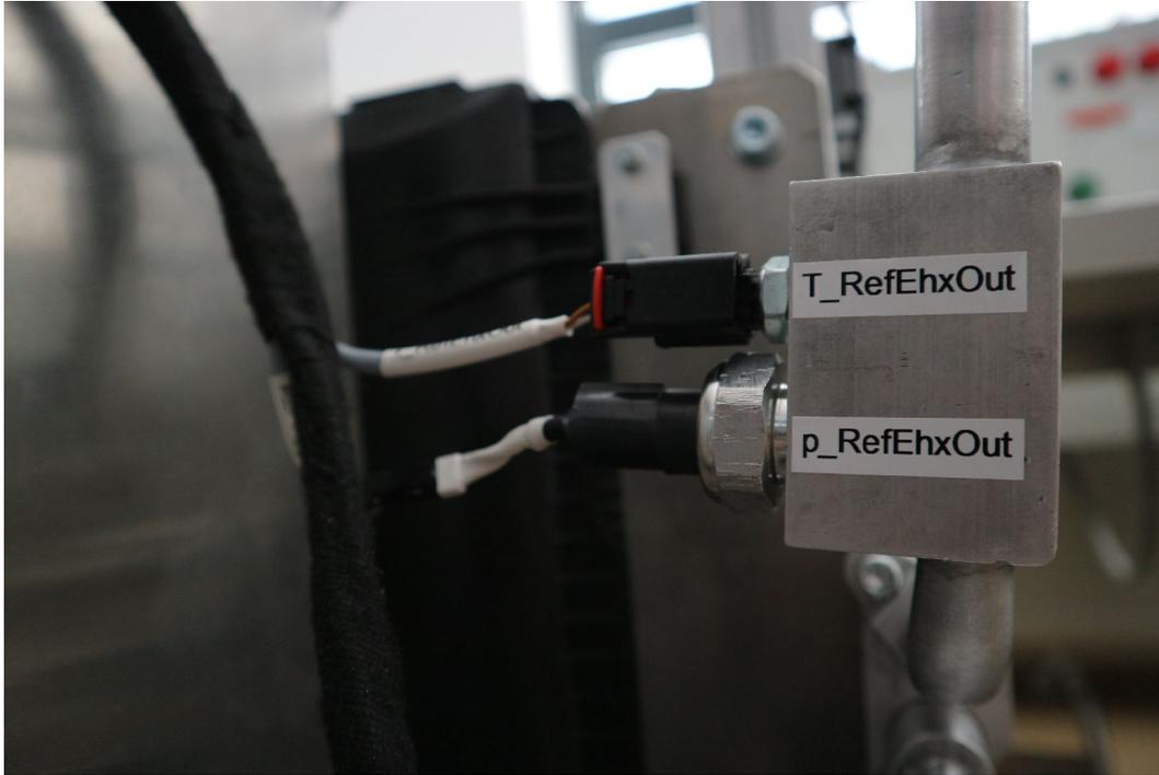
Fig. B.9: Refrigerant temperature and pressure sensors
