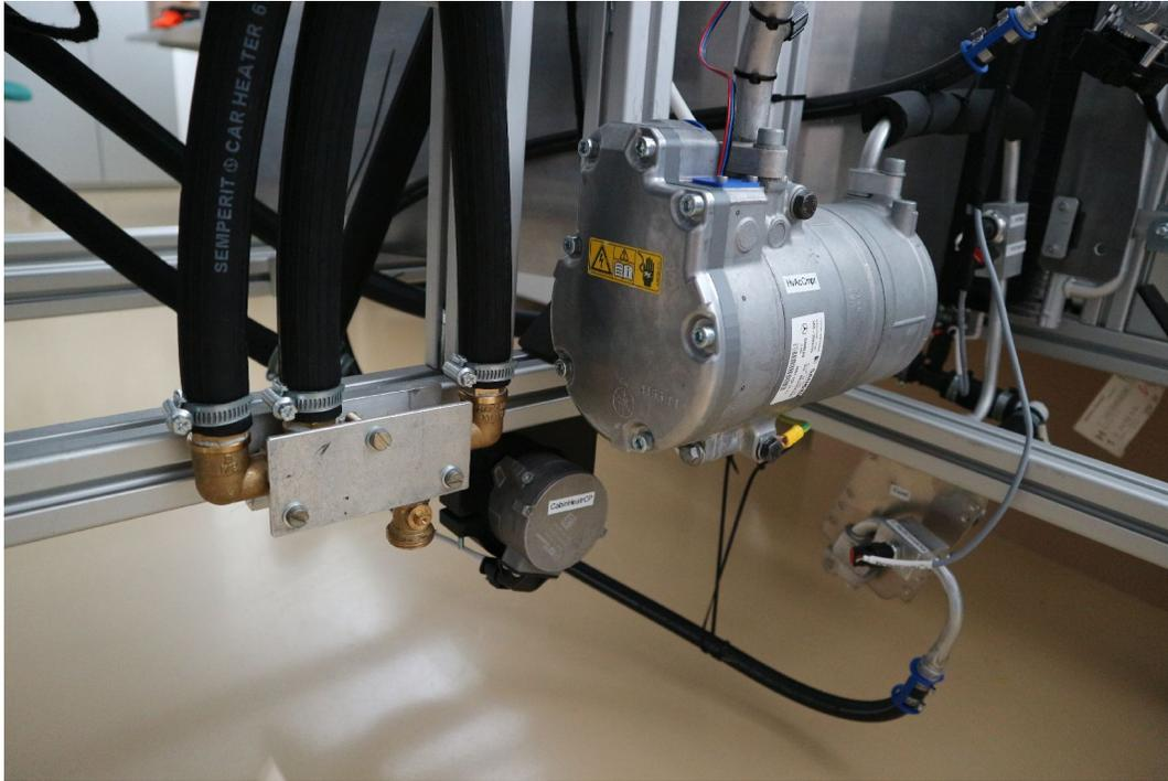
Fig. B.5: HV compressor and coolant pump
